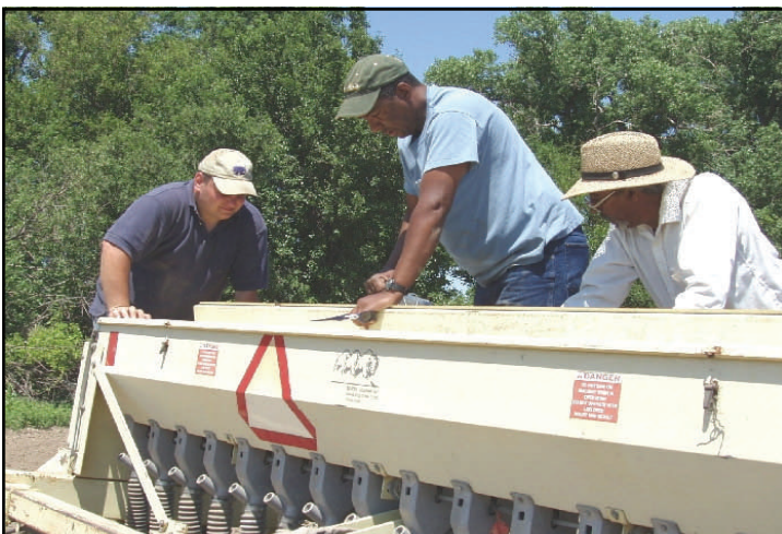
Project Coordinator, Josh Coltrain, and teff producers Gil Alexander and Gary Alexander adjusts the drill settings for the small teff seed.
